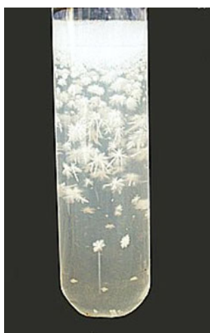
Fig. 1 Star shaped lead iodate crystals inside the gel medium
