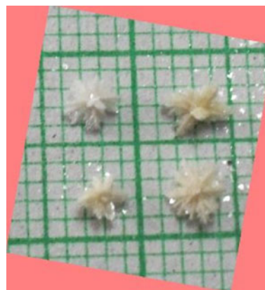
Fig. 2 Star shaped lead iodate crystals outside the gel medium
